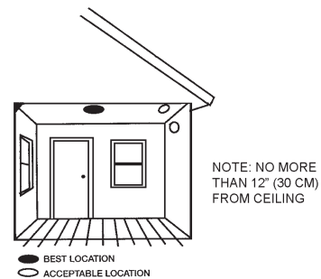
FIGURE 5: RECOMMENDED SMOKE ALARM MOUNTING LOCATIONS
